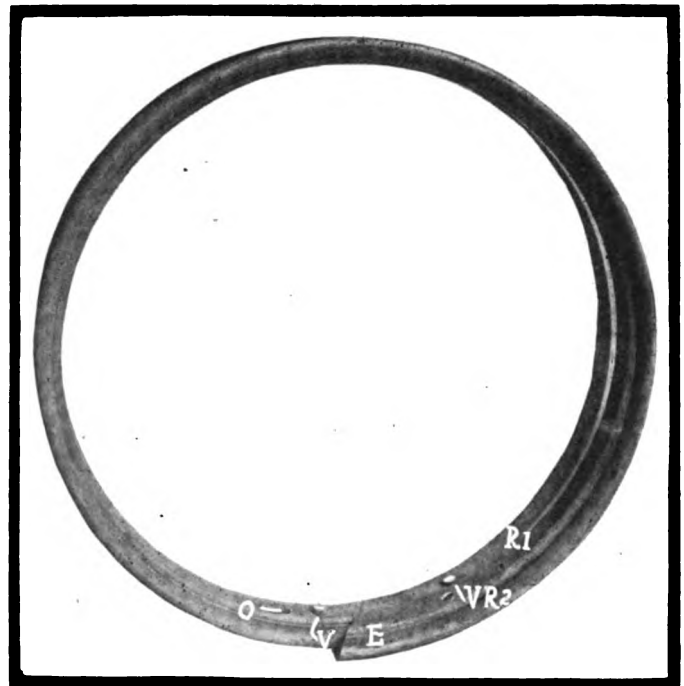
Fig. 3—J-M demountable rim, shown off the wheel, illustrating the use of two rings and two-stud scheme
